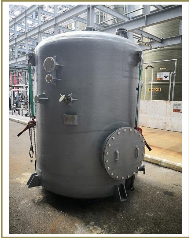
Chemical decomposer tank
