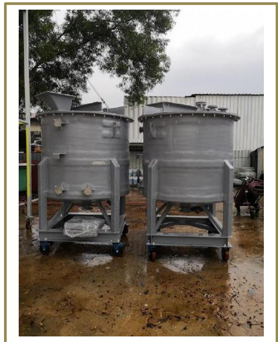
Chemical storage tanks undergoing hydrostatic test
