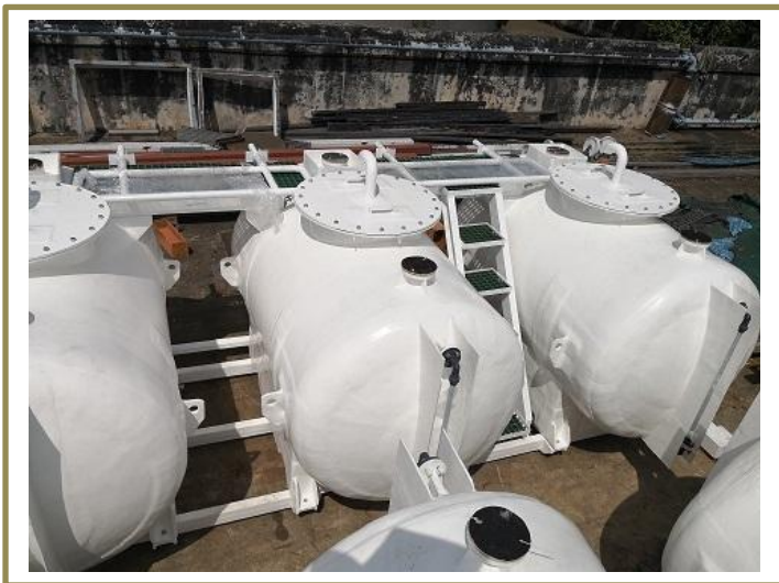
Sodium Hypochlorite storage tanks incorporated with skid, ladder, platform and foldable hand rail
