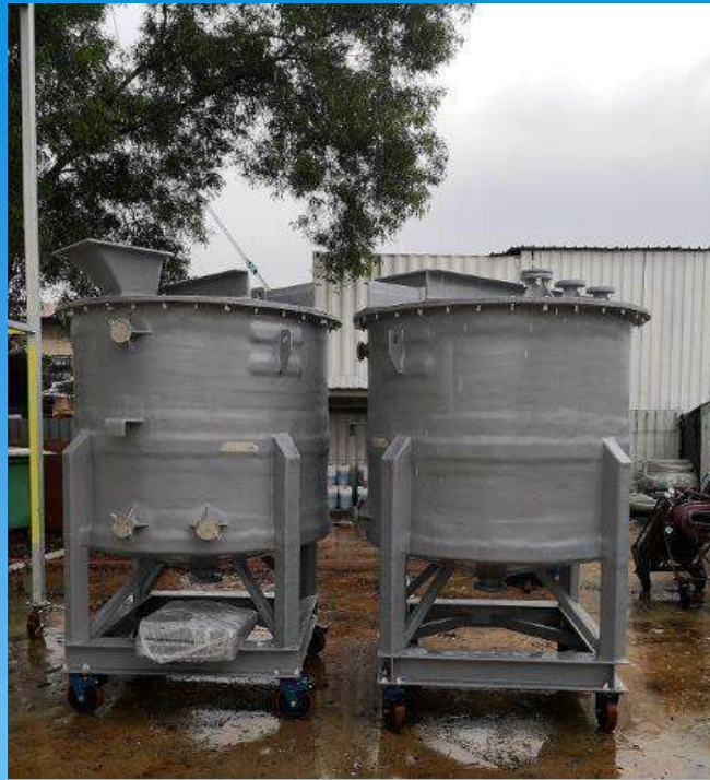
Skidded Mixing Tanks
