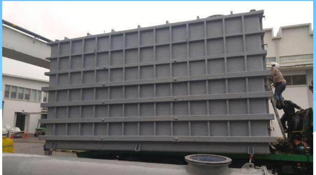
Waste Water Holding Tank
