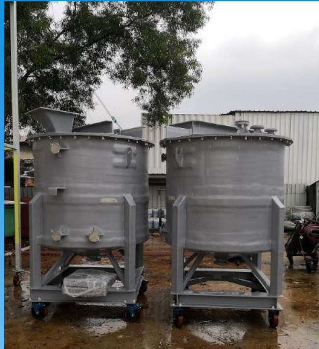
Skidded Mixing Tanks
