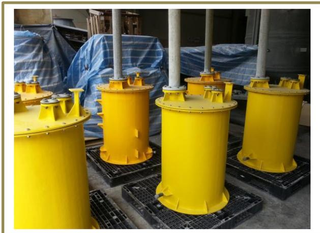
**Chemical storage tanks undergoing hydrostatic test**
